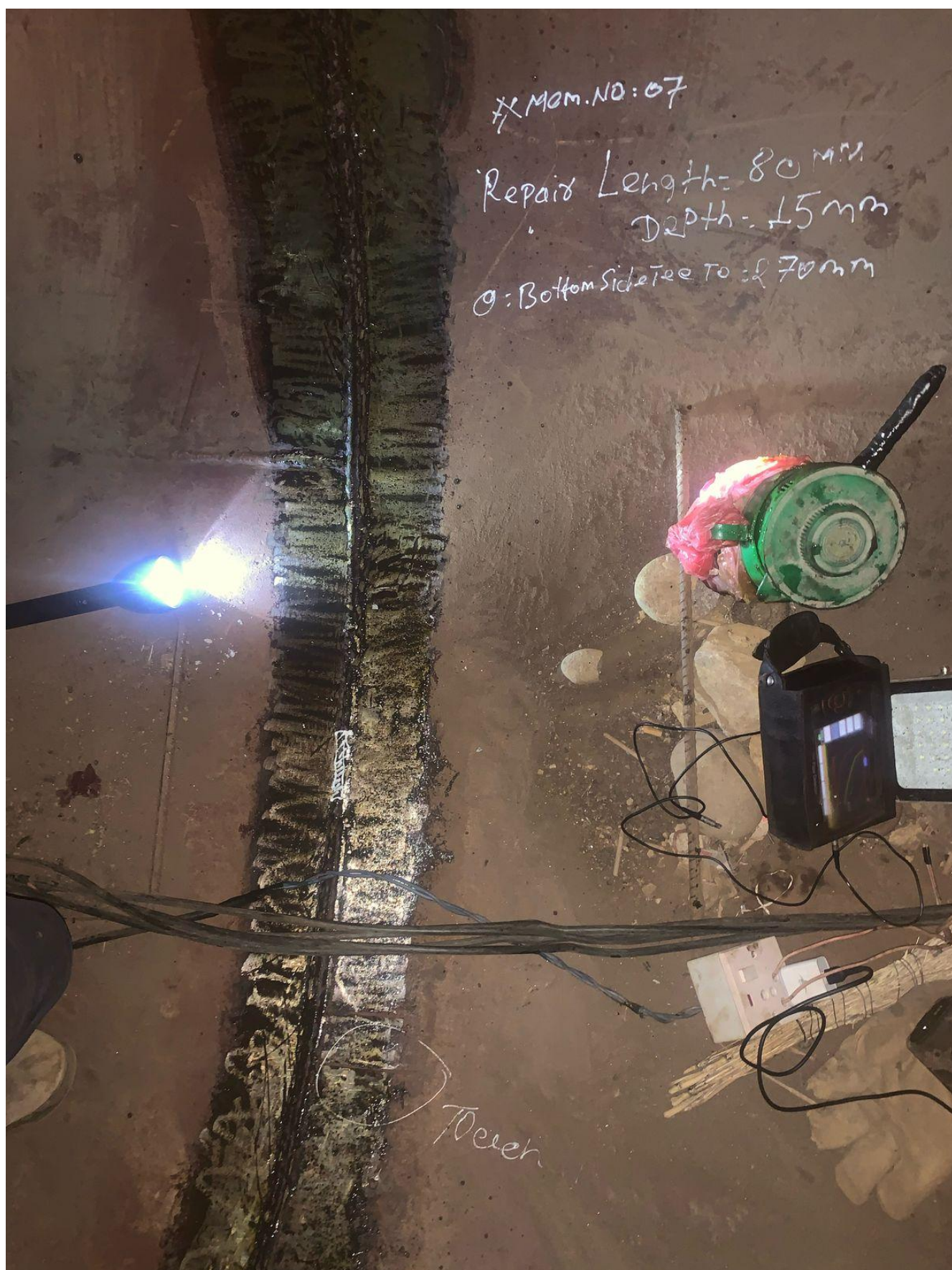
Figure 18: Ultrasonic test of welding at penstock pipe.
