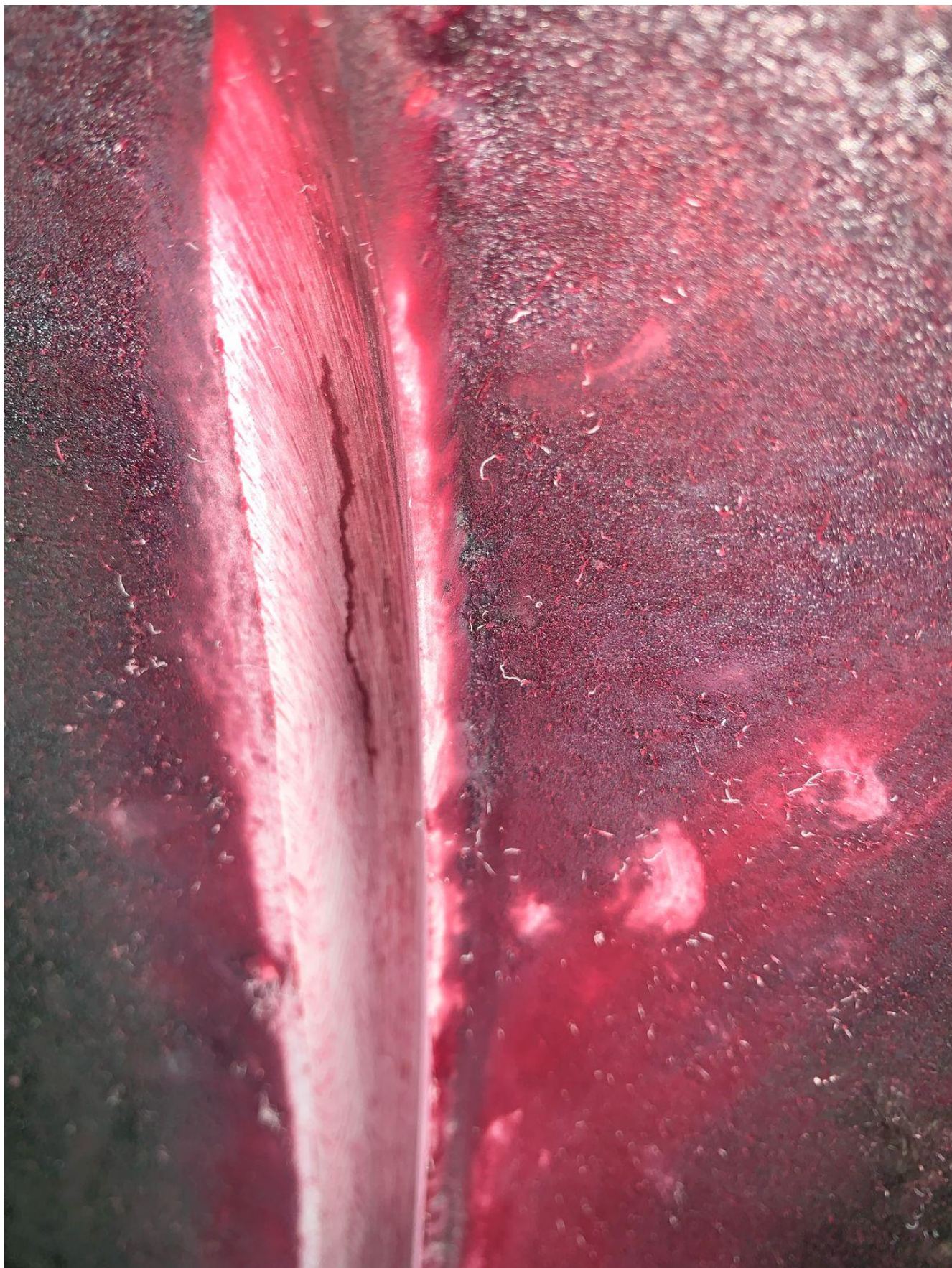
Figure 19: Ongoing Dye Penetration test of welding at headrace and penstock pipe
